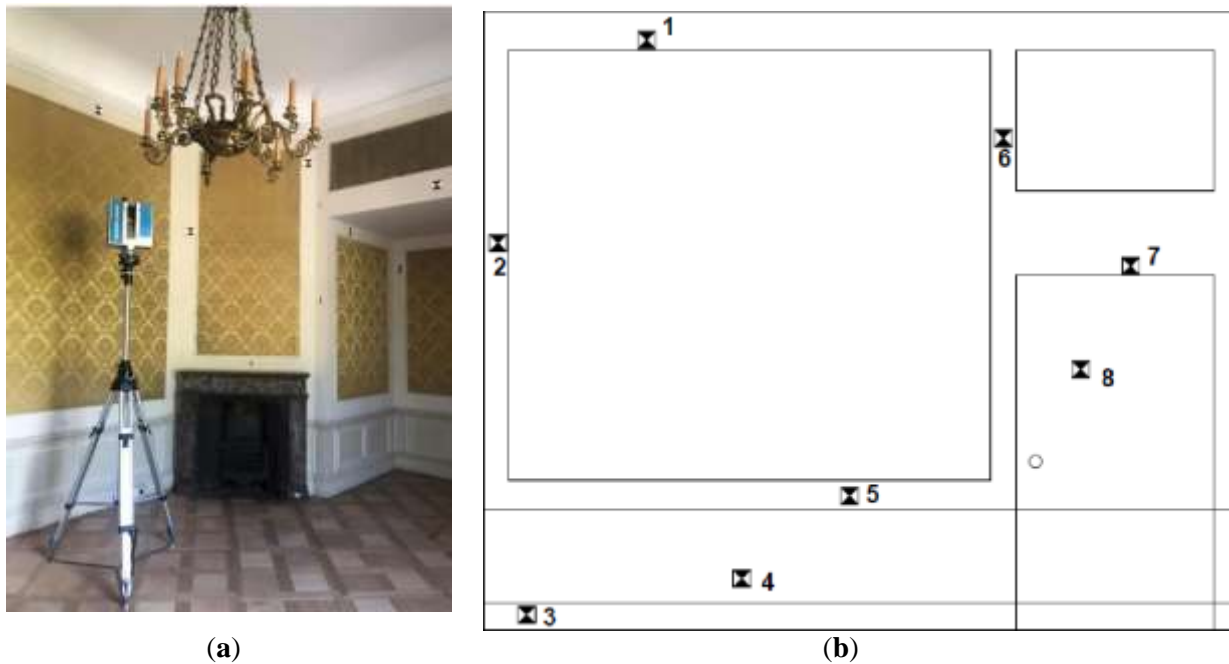
Figure 3. (a) Room section with visible points on the walls and with the Z+F Imager 5006h scanner, (b) The sketch of one of the walls with the location of the control/check points.
