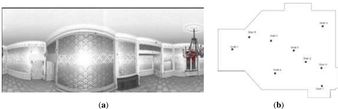
Figure 4. (a) The example of a point cloud in spherical projection, (b) The sketch of scanner stations.
